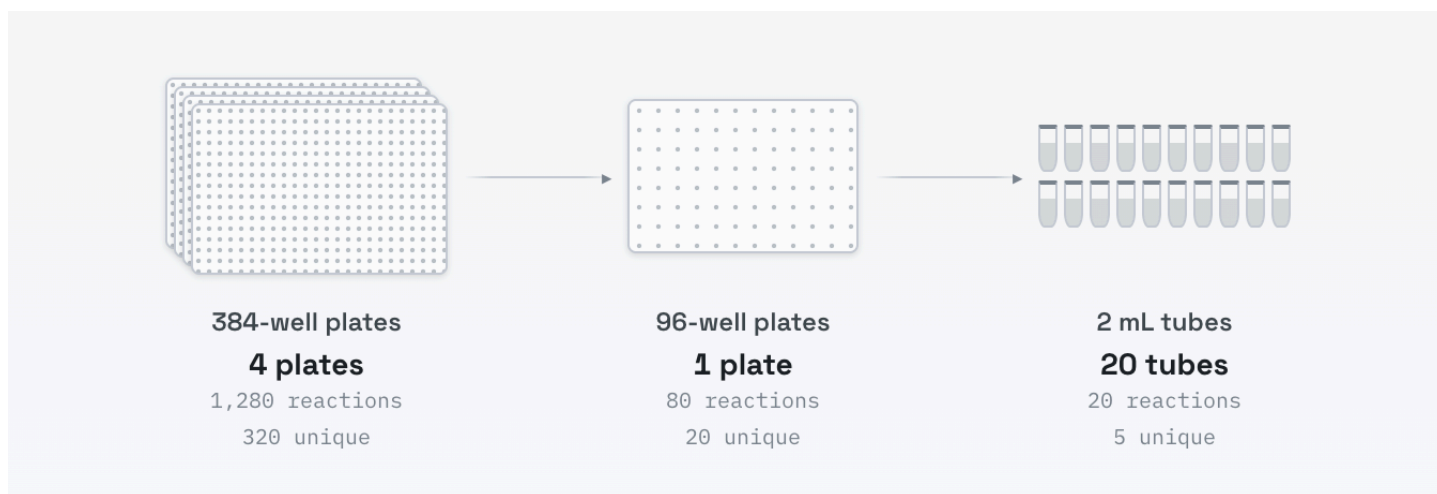
Fig 1. Ginkgo's staged screening strategy. Testing begins in 384-well plates with best CFPS compositions further evaluated in 96-well and 2 mL tubes
